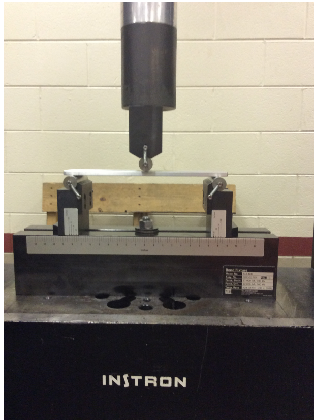
Figure 3: Bending Test (Before)
