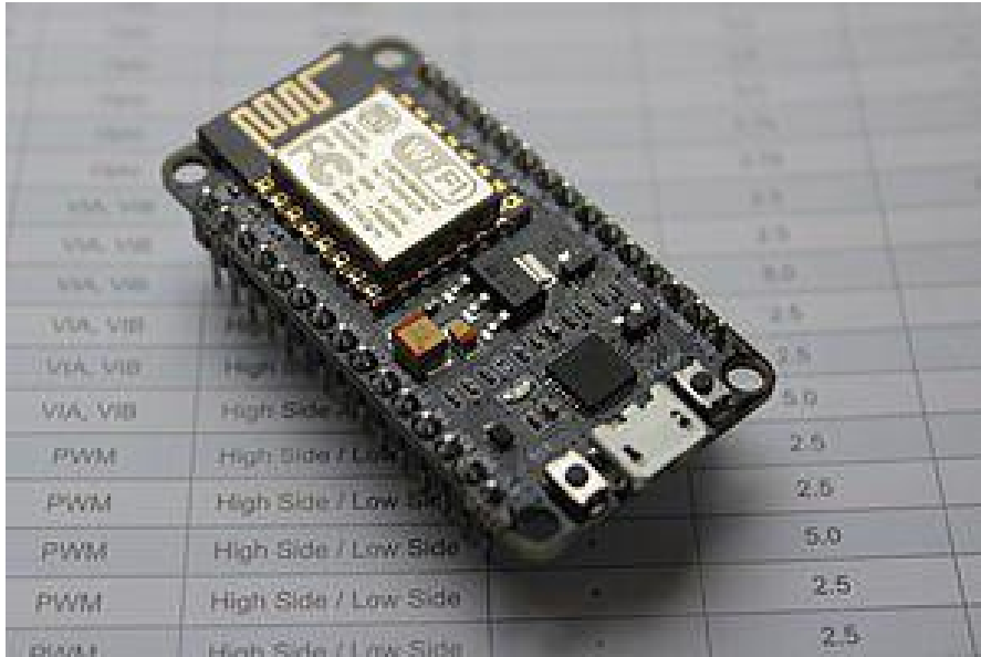
Figure 2.1: NodeMCU Chip Diagram
